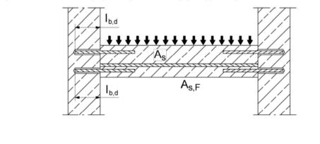
Rebar connection with fischer injection mortar FIS V
