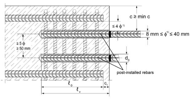
$<sup>^{1)}</sup>$  If the clear distance between lapped bars exceeds 4  $\phi$  then the lap length shall be increased by the difference between the clear bar distance and 4  $\phi$
