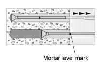
Insert injection adapter to back of the hole. Begin injection allowing the pressure of the injected adhesive mortar to push the injection adapter towards the front of the hole.
