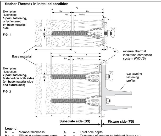
$h_{ef}$  = Effective embedment depth e = Thickness of layer to be bridged ( $t_{WDVS} + t_{tol}$ )  $t_{fix}$  = Fixture thickness  $t_{tol}$  = Thickness of old plaster and/or adhesive U = Overhang  $\geq 1 \text{mm}$   $t_{WDVS}$  = Insulation thickness (system)
